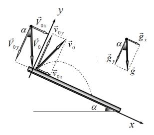
$$V_{0x} = V_0 \sin \alpha$$
